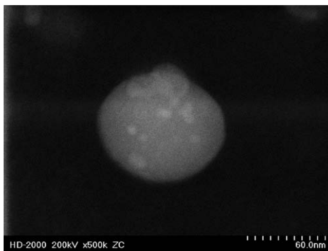
Figure 4. TEM analysis. Cellax particles were applied to Formvar coated copper grids, and analyzed by dark-field TEM (500 000× magnification). Six randomly picked particles were imaged, and the size was measured: particle diameter = 104 \pm 15 nm.
