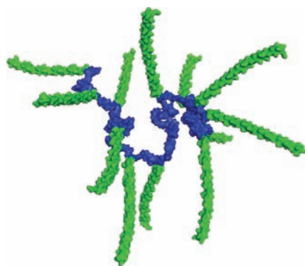
Figure 5. Schematic representations of rAFP-N/PAA reaction product. The rAFP-N models were created by extending the length of winter flounder AFP (PDB ID 1WFA 37 ) while maintaining the \alpha -helical structure, using DeepView/Swiss-PdbViewer software program. 38 PAA (17 kDa) was produced using PyMOL version 0.99.
